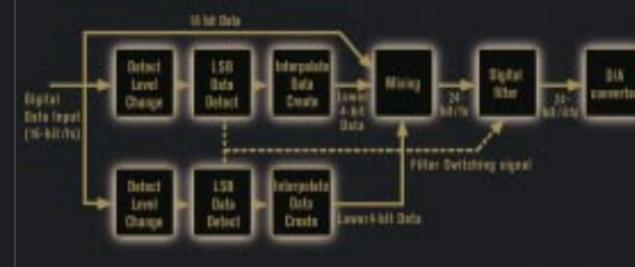
from becoming distorted during peak periods, and boosts the low-level signals to improve the S/N ratio for a substantially richer dynamic range.
