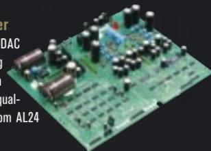
Processing with utmost fidelity. This design achieves a signal-to-noise (S/N) ratio of 118 dB and a dynamic range of 108 dB, to bring out the beautiful sound of high-bit, high-sampling technology.
